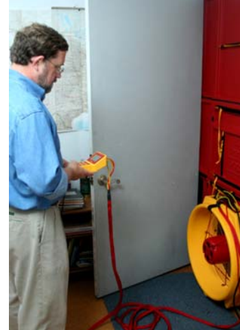
Performing a Blower Door Test
